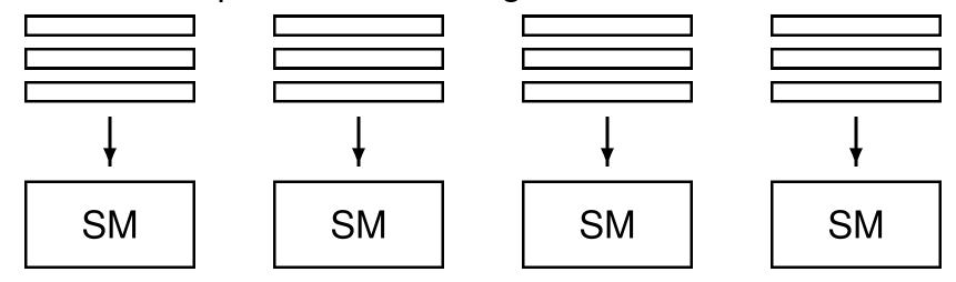
In this simple case, we had a 1D grid of blocks, and a 1D set of threads within each block.
